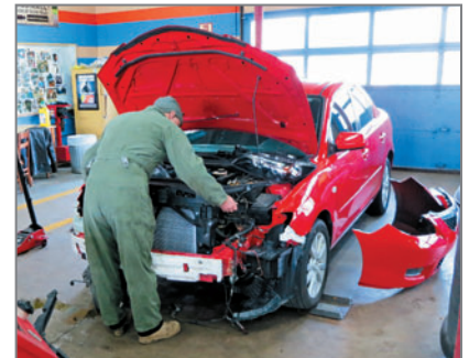
This Mazda kind of took it on the chin from a concrete post. While the repairs were fairly simple, the parts were expensive – particularly that plastic radiator support, which had to come from the dealer.
