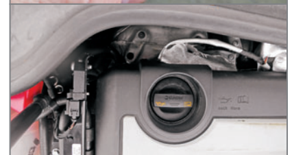
The 2009 Jetta had a bad EGR pressure sensor – a remote relative of the DPFE sensor on Fords, only this diesel has two sensors. The funky foil wrap right behind the oil filler cap hides the sensor we replaced. Note the identical sensor at the end of the engine.
