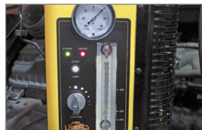
The Smoke Wizard features a pressure/vacuum gauge, flow meter and flow control.
