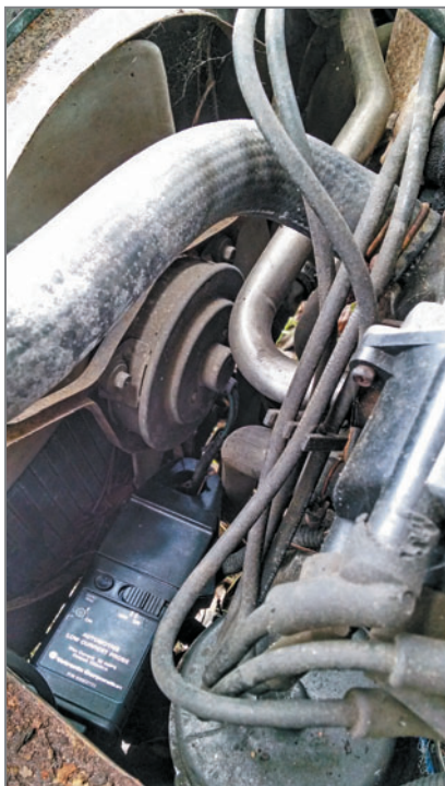
Considering everything else had been replaced without success, I thought a test of the cooling fan motor condition was in order.
