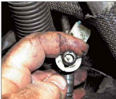
You can get better smoke and pressure flow by optionally removing the left-hand thread Schrader valve in the test port.
