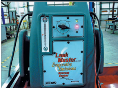
Smoke is emitted for a few minutes at a time on this machine before timing out. Be sure to follow OEM recommendations for using CO 2 or nitrogen for system testing to avoid fire/explosion hazards.
