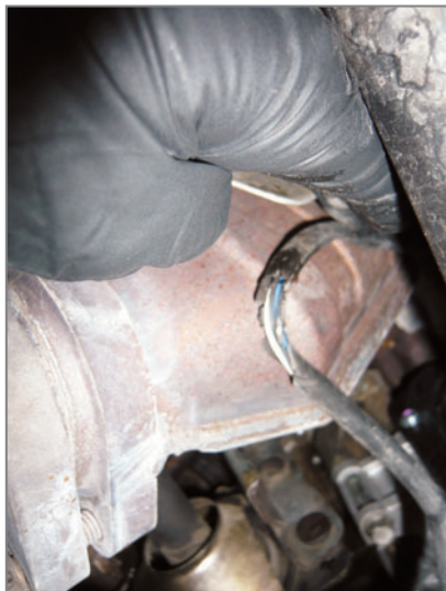
This was the cause of Code P0037 HO 2 S Heater (Rear, RH) Circuit Low, the wires fell from the wiring harness retaining loom and melted on the exhaust.
