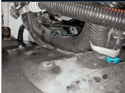
With the harness supported, there was just enough electrical contact to allow the truck to run and the scan tool to communicate. It's a perfect example of the importance of voltage drop testing.
