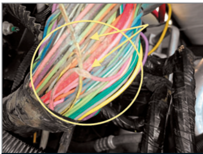
Only a few strands remained intact on the PCM ignition feed wire.
