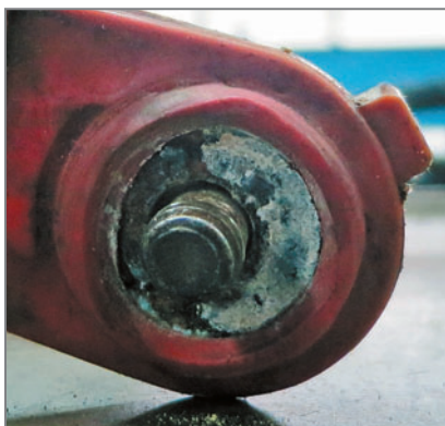
This was causing the Malibu's intermittent no-crank. Replacing the battery did nothing to solve the real problem, so we replaced this cable with a new one.
