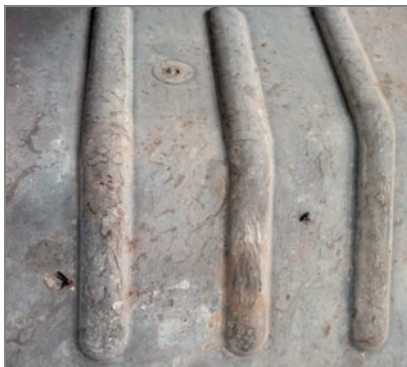
With the inner fender removed, the signs of harness contact were easy to see.
