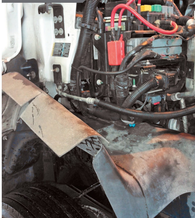
You can see the inner fender is partially installed, and how the skirt supports the weight of the harness.
