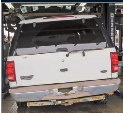
This Expedition had a flat air spring; the one on the right had been replaced right before it was parked. We sold them on replacing the rear suspension with coil springs and the kit came with a full set of shocks. This SUV went from being parked to getting a new license plate and lease on life, but not before we replaced the leaking brake pressure switch for safety.
