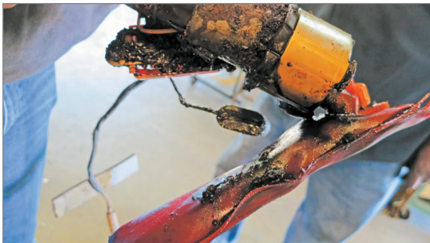
When we got the gas tank off the 626, we found this disaster, along with another 30 pounds of the same gunk in the tank.
