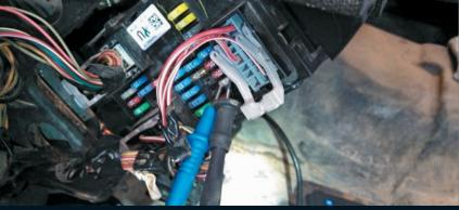
Testing volt drop across the 25-amp rear wiper fuse on the Suburban.
