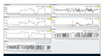
Here is fuel trim data taken at 2,500 rpm. The long term has changed to -10 on bank 1 and +20 on bank 2. Short trims still look normal. Again, this problem has been around long enough, so all the short-term corrections have been moved to long term.
