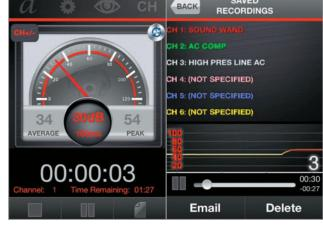
hear under the hood or chassis. The Smart Ear 1 app comes with an equalizer, so the user can zero in on specific pitches and frequencies of noises. Applications include, but aren't limited to, finding fuel injector misfires, loose bearings in an A/C compressor, or pinpointing noises in differentials, idler arms or tie rods.
