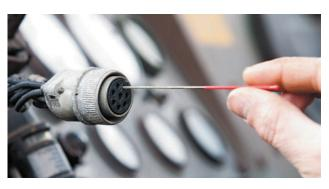
terminals in the industry, and are designed to precisely scrape corrosion from both male and female pins without damaging the integrity of the terminal.
