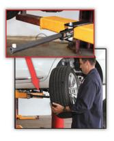
in 10 minutes and with a 100-pound capacity is capable of holding the heaviest passenger car and light truck tires, according to the manufacturer. Heavy rubber coating on the Backsaver prevents damage to expensive wheels and rims.
