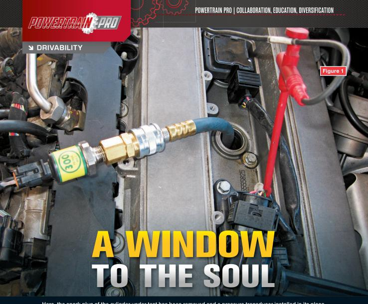
Here, the spark plug of the cylinder under test has been removed and a pressure transducer installed in its place.
