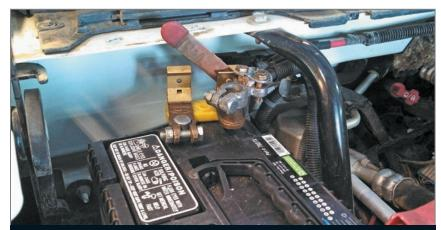
Here is a high-amp switch installed on the negative battery terminal. This switch is used so the vehicle can be started and driven. The meter test leads are then hooked to both sides of the switch, then the switch is open. That allows the current to flow through the recording meter, and allows the meter to be hooked up without disrupting the power to the vehicle.
