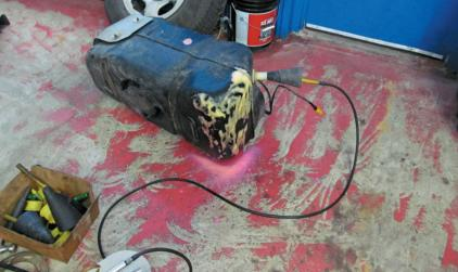
The BullsEye leak detection system uses CO<sub>2</sub> and a special foam agent that changes color in reaction to the gas to help find the most difficult leak. Here, the tank is porous and leaking over a large area, which is an unusual case found easily with new techniques.
