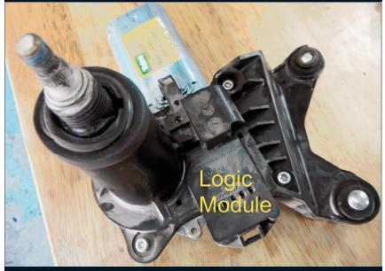
This is the rear wiper motor/module and the logic module. This window motor works normally, and the only problem is the 0.6 amp draw - which will kill the battery if the vehicle is not driven every day.
