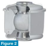
MOOG's patent-pending new Problem Solver control arm bushings (see Figure 1) for vertical applications feature an innovative balland-socket design (see Figure 2) that eliminates stress-induced failures encountered in original equipment-style parts. Lasting up to 10 times longer than original equipment (OE)-style parts, these new MOOG bushings are available for millions of popular Chrysler, Ford, General Motors, Honda, Mazda and Toyota passenger vehicles.
