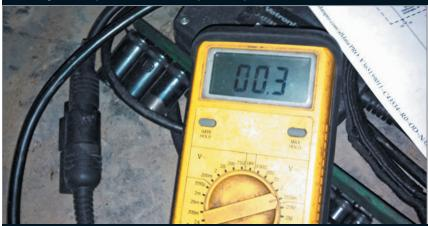
Here are the results of the volt drop test across the 25-amp rear wiper fuse. The volt meter shows 0.3 mA of volt drop. This fuse is flowing 0.6 amps of current.
