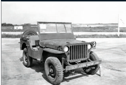
Willys MB test vehicle with stamped metal grille designed by Ford.
