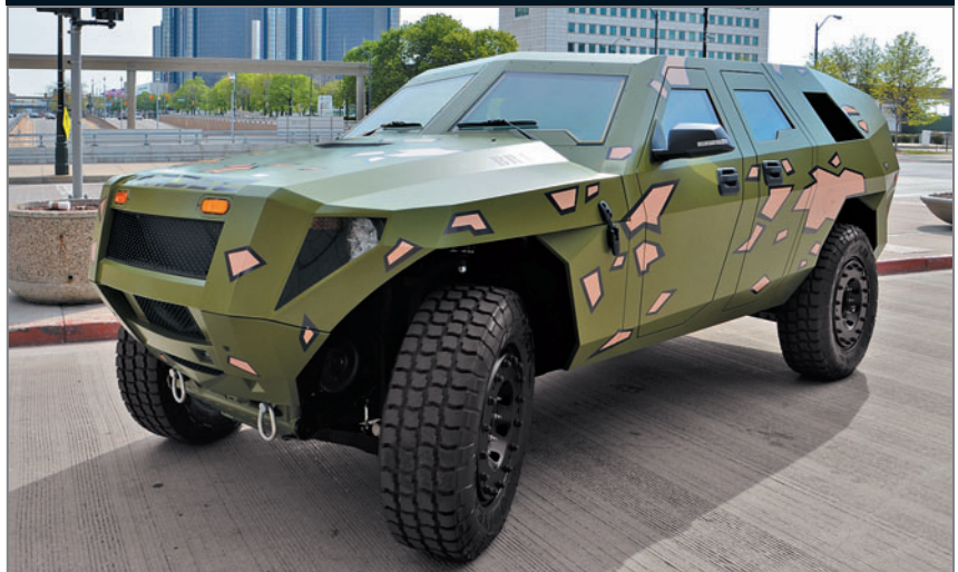
The FED Bravo added a hybrid system to the FED Alpha, plus the ability to export electrical power for field use.
