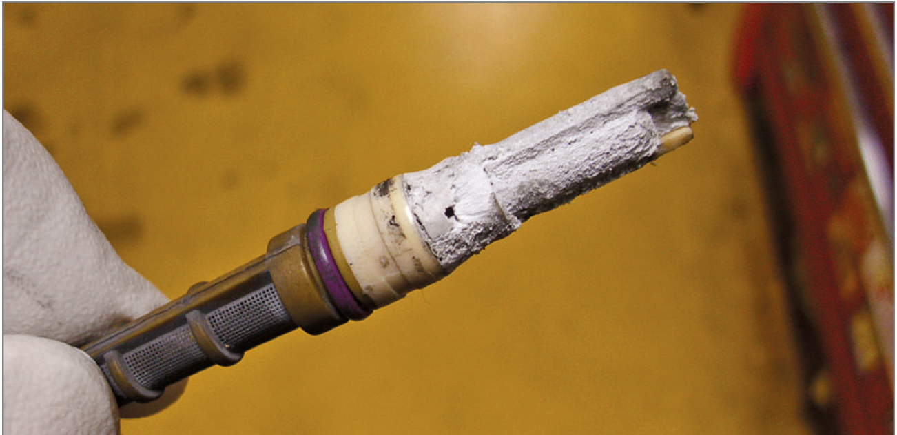
Sealant is a leading cause of compressor failures and system woes.
