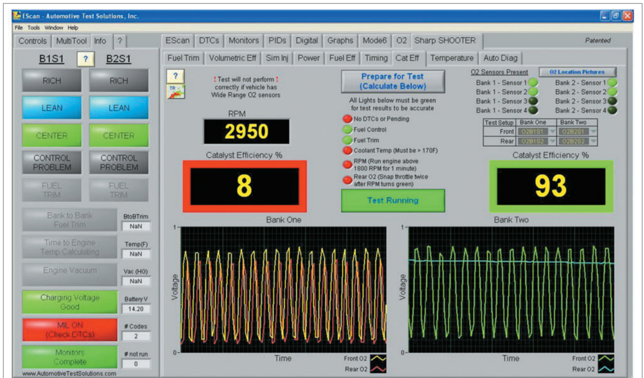
Checking the efficiency of two cats at once. Notice how the two O 2 sensor patterns on the left mirror each other (bad), while the two on the right are an example of a properly working converter.
