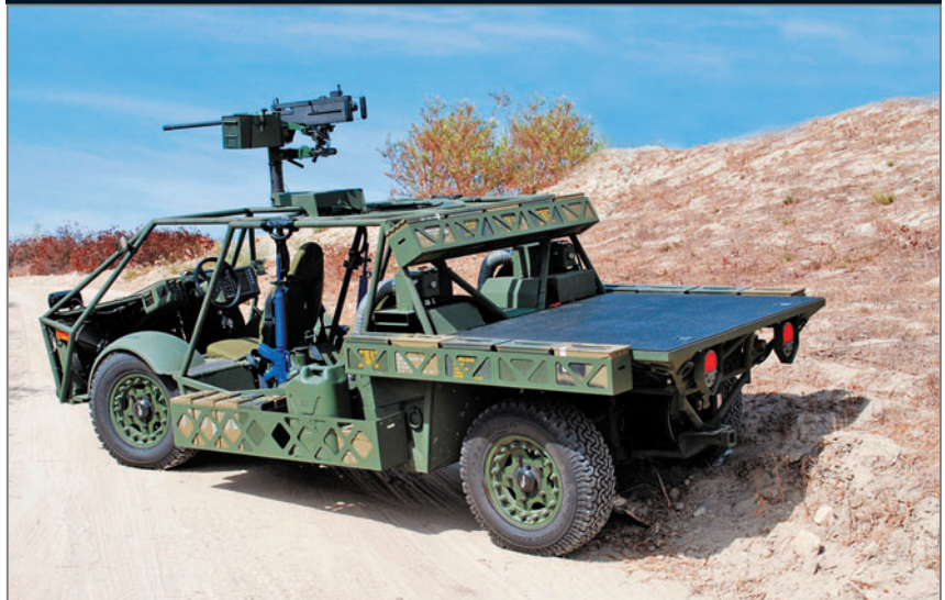
The CERV uses electric drive and can go silent (electric only) for up to 12 miles.
