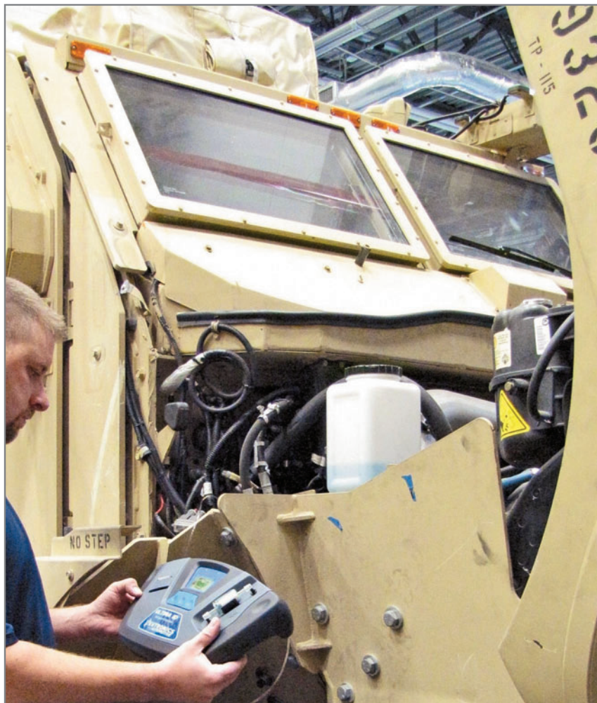
TARDEC Senior Engineer Jeffrey Marcinok uses a refrigerant identifier to field test a vehicle.
