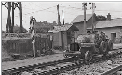
Willys MB Jeep rigged to run on railroad tracks.
