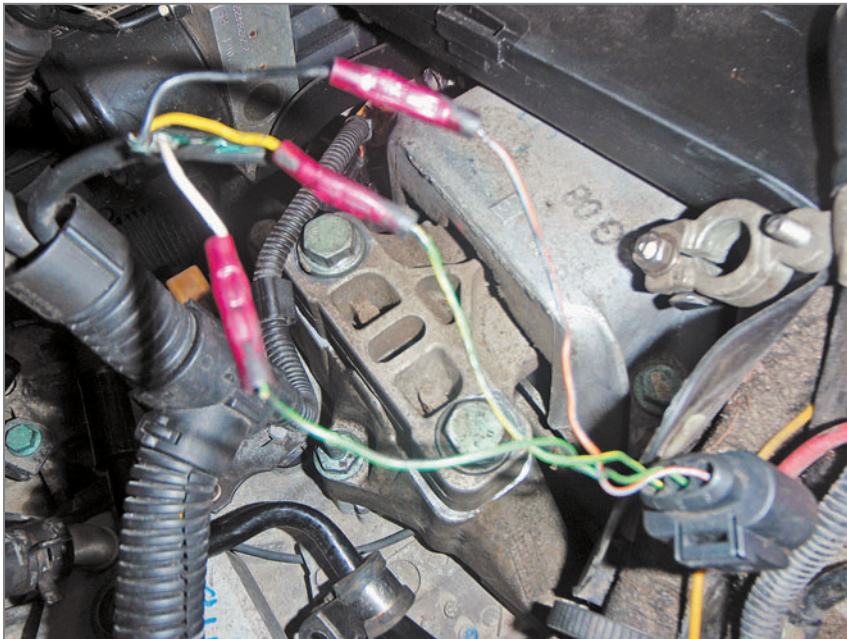
Here is the G68's new harness connector that someone already tried. Note the wire color change.
