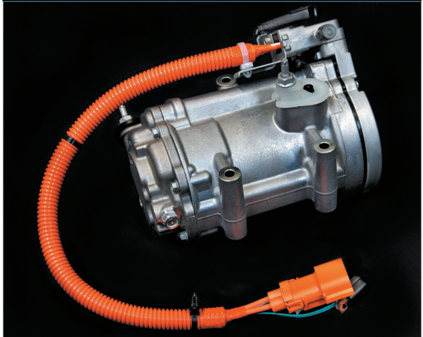
A high-voltage A/C compressor is identifiable by the orange wire loom.
