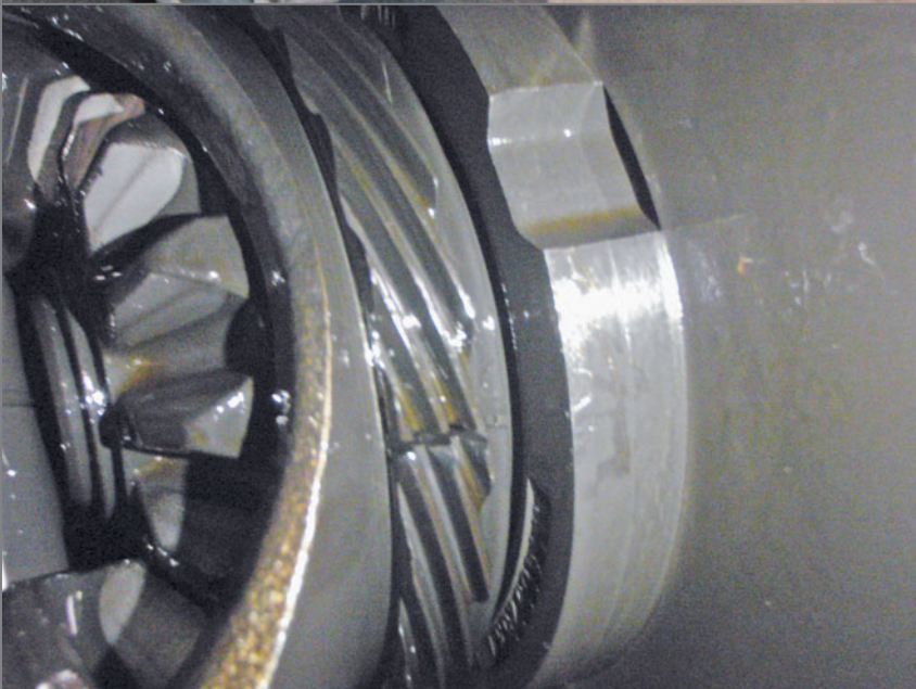
These images are of the transmission after it was removed. The differential side cover was removed for reference of the speed sensor to drive gear relationship. Also, the crack can be seen with the sensor removed.
