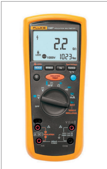
An insulation tester such as the Fluke 1587 may be necessary to diagnose HV insulation faults.
