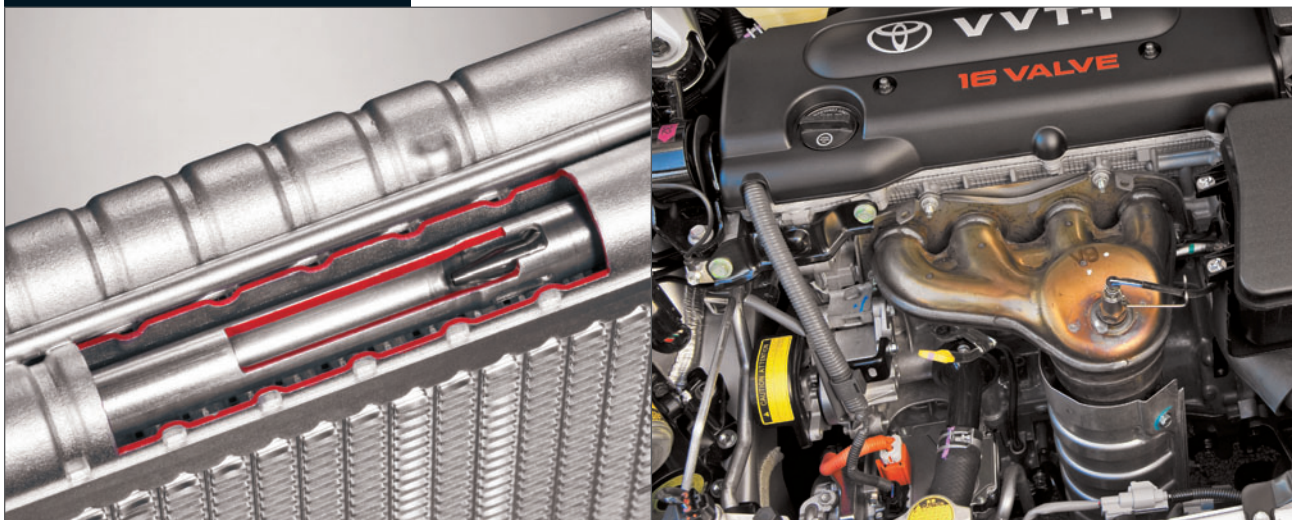
(Left) A cutaway look at the ejector. (Right) The orange HV cable to the A/C compressor on this current-generation Toyota Hybrid has high-voltage DC sent to the compressor where it is inverted to A/C to drive the motor.
