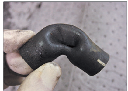
This failed PCV elbow is all it takes to cause a lean idle condition. Smoke from your EVAP tester, though, makes them easy to find.
