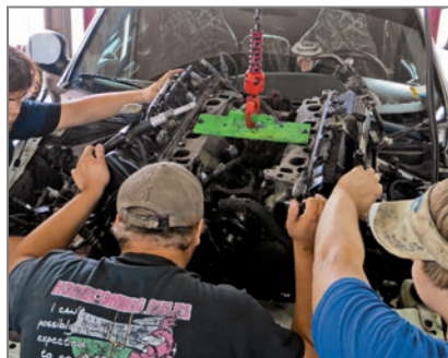
Here was the original engine coming out. Some techs raise the body off the frame to do this, and Willie opted to remove the transmission first – both times.
