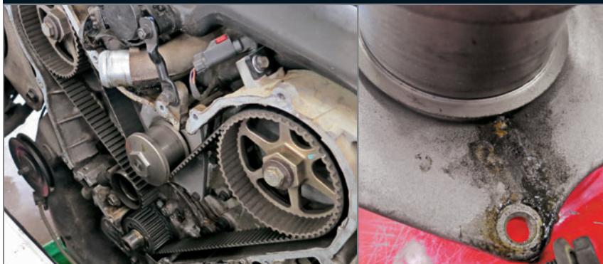
Here is the 300 with its leaking water pump. Garrett managed to break one of the 6 mm water pump bolts off and had to center drill and work the broken piece back out of the aluminum housing with an extractor. It was pretty dicey on a bolt that small at that angle.
