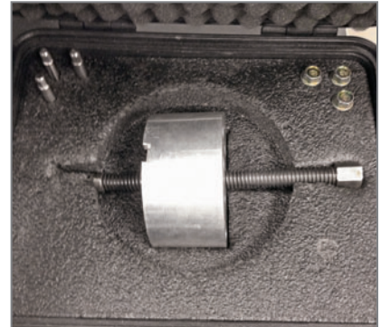
IMA rotor removal requires a special pulling tool and includes a case to store the rotor while it’s removed.
