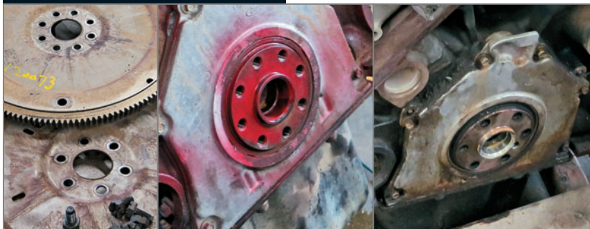
This flywheel issue kind of blind-sided me. I wondered briefly if we had received a Windsor engine instead of a Romeo, because the crankshaft and flywheel must have come from two different vendors in that year model F150.
