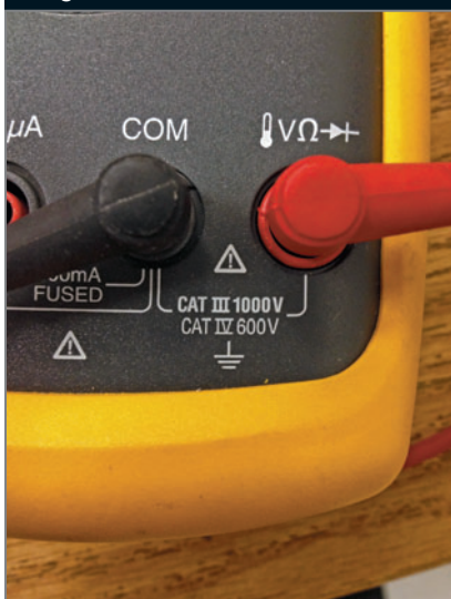
Be sure your meter is rated for high voltage.
