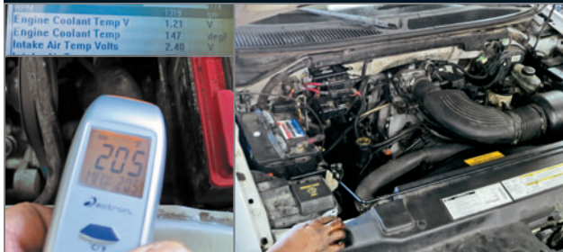
(Left) This situation grew from a P0128 code on a 2006 Mountaineer that came in while the F150 was there. The engine was running at normal temperature, but the ECT sensor was reading about 50 degrees cooler than the truth. (Right) Willie was making his final tweaks here, and the owner took possession of the truck the next morning. It had been one grand adventure.
