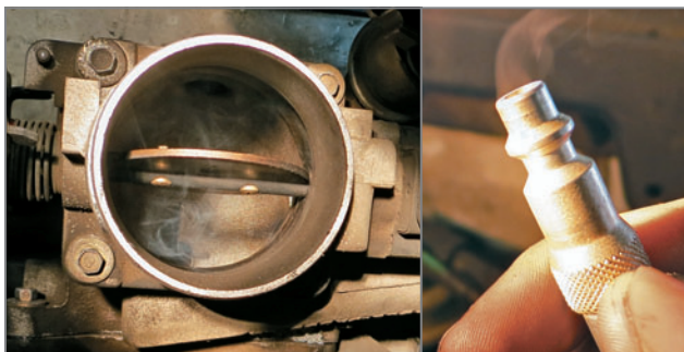
This tattletale smoke trace from our Evap Tester pointed to a compromised intake valve. Capping the intake and pumping smoke into it wafted smoke out the feed fitting, too.
