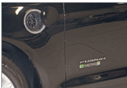
A sign of times to come: Not a gas door, but an electrical connection for direct charging of the HV battery pack.
