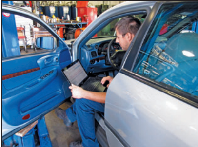
Mike Barran checks an oxygen sensor output voltage on laptop.
