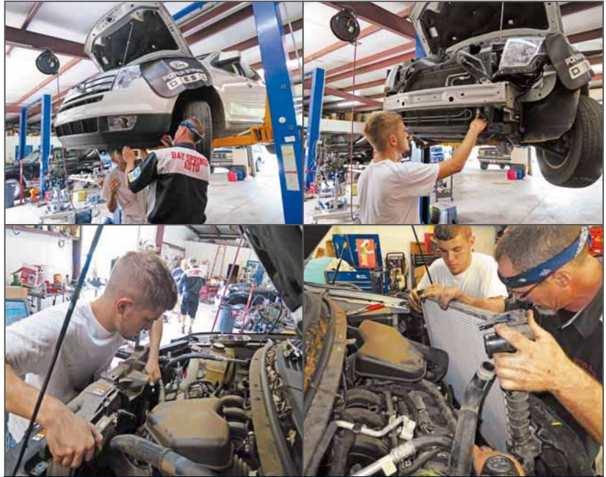
On the Edge, after recovering the refrigerant, the fascia had to be removed. The coolant the was drained and the fan and radiator/condenser package were removed so as to access the receiver/dryer sock. This is a TXV system, but there was no reason to change it for an external compressor failure.
