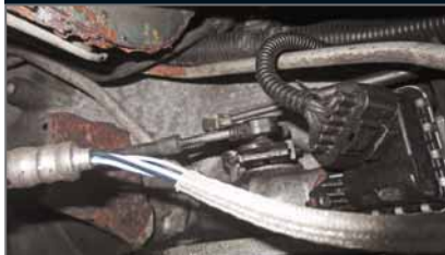
Even though this cable had popped off, the shifting problem wasn't corrected until I fixed the O 2 heater code.
