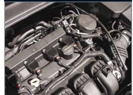
Ford has clearly shown you what weight of oil to use, no mystery here.
