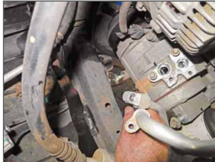
To remove the compressor, the bottom stud had to be screwed out of the mounting boss and removed with the compressor, which, in this case, showed signs of electrical coil failure. It didn't blow the fuse, but it got plenty hot enough to do this, and all the customer had was a blower moving hot air.
