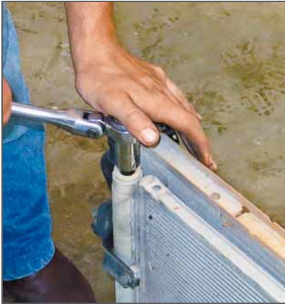
To remove the compressor, the bottom stud had to be screwed out of the mounting boss and removed with the compressor, which, in this case, showed signs of electrical coil failure. It didn't blow the fuse, but it got plenty hot enough to do this, and all the customer had was a blower moving hot air.
