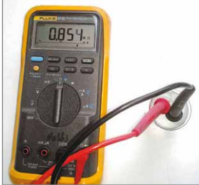
Suspect alcohol in the fuel? Put your ohmmeter leads in it. Any reading indicates alcohol, since it is conductive while pure gasoline is dielectric.
