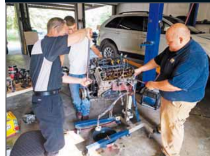
This 2001 4.0L Explorer engine requires a lot of torque-to-yield work on the jackshaft and camshaft bolts and a bevy of special tools to keep everything locked in and in line.
