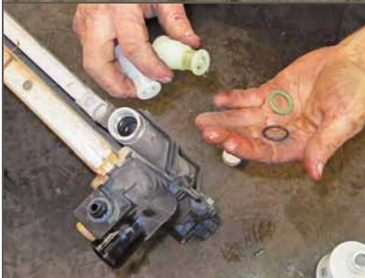
Flipping the radiator and condenser upside down, it took a 14 mm Allen wrench to get this plastic filter plug out and some mechanical fingers to grab the sock. The new plug looked right, but wouldn't fit. Donnie used the new O-ring and the old plug. This kind of misfit happens a lot more than it should.
