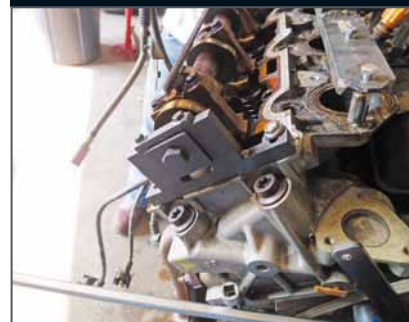
This 2001 4.0L Explorer engine requires a lot of torque-to-yield work on the jackshaft and camshaft bolts and a bevy of special tools to keep everything locked in and in line.
