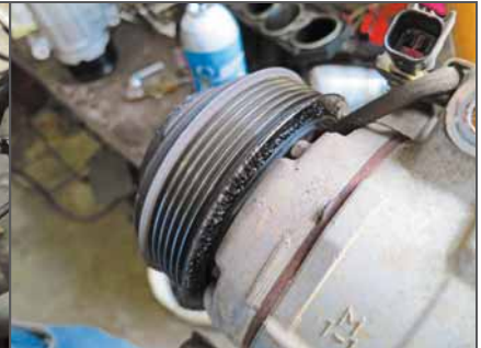
To remove the compressor, the bottom stud had to be screwed out of the mounting boss and removed with the compressor, which, in this case, showed signs of electrical coil failure. It didn't blow the fuse, but it got plenty hot enough to do this, and all the customer had was a blower moving hot air.
