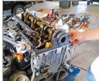
I don't have a photo of the tool that locates the crankshaft at No. 1 TDC, but the tool at the top locates the camshafts and the tool at the bottom holds the gear securely during the torque-to-yield process. The bolt on the right rear gear is left hand thread, by the way.
