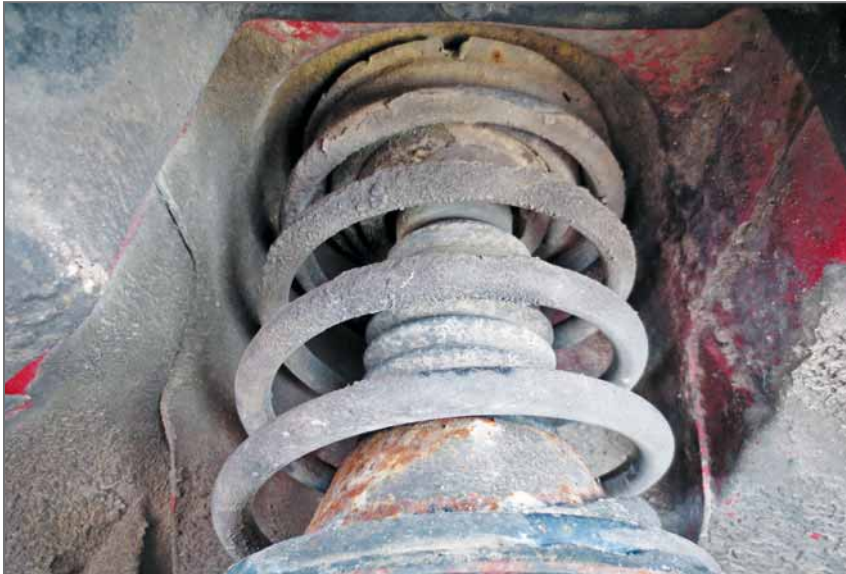
Check the struts for broken springs, leaks, and components that aren't where they should be.
