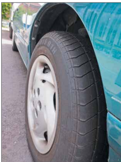
Sometimes rough tire wear patterns are really obvious. The edge of this tire feels like it looks: rough.
