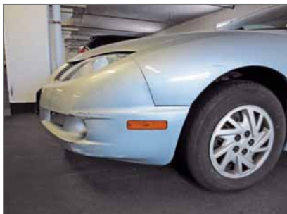
Look for signs that the vehicle has been involved in an impact.
