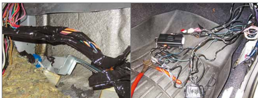
(Left) Not an every day occurrence, but not uncommon either. Failed seals can allow fluids to wick up wiring harnesses for a surprisingly long way. (Right) A professional remote starter installation – or maybe not.
