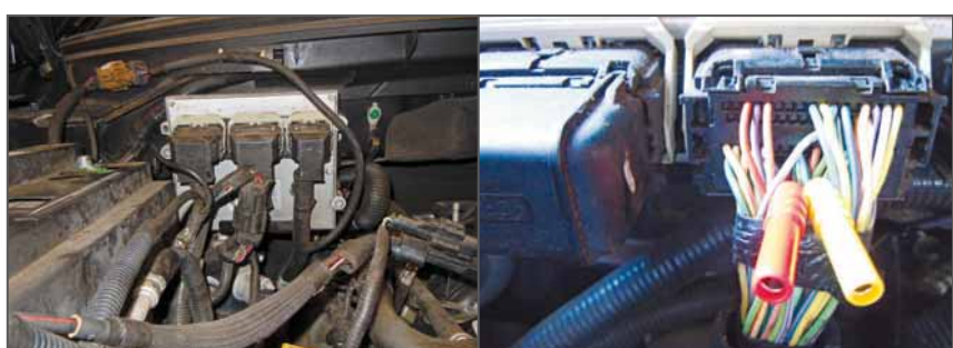
(Left) The PCM connectors have unique purposes. The connector on the far right is called Connector "E" (Engine), the center one is called "B/C" (Body/Cowl) and the far Left connector is called "T" (Transmission). (Right) In order to test the Knock Sensor(s) and their circuits, one must back-probe the PCM Engine connector after disconnecting it from the PCM, then read the resistance between pins E48 and E49 (KS1) or pins E30 and E31 (KS2). Resistance tests are the only component tests found for these sensors. There wasn't much room for the back-probes as seen in this image.
