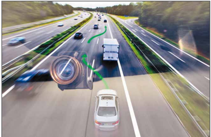
The onboard camera can detect approaching traffic and even be used to monitor how well the car is staying in its lane.
