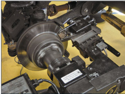
Using an on-car brake lathe is one way to ensure that the pads ride true to the rotor surface.
