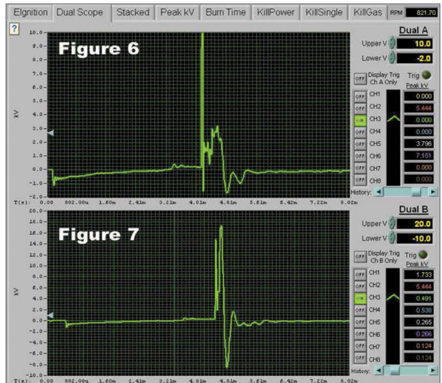
A lack of fuel alters the composition of the plasma channel.
