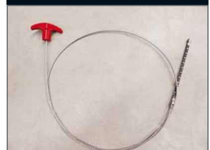
This is the tool used to check Chrysler and Daimler products that have a tube but no dipstick.
