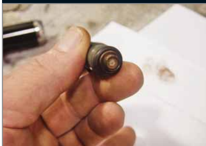
Even a slight restriction to fuel flow can cause a no code drivability complaint.
