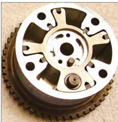
Vane-style is the most common design for a VVT actuator. Locking pins can become stuck due to lack of proper oil maintenance.
