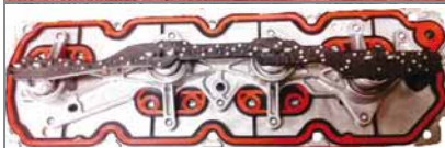
This GM system can be tested much like you would a transmission valve body.
