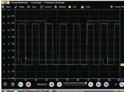
Most OEMs use crank speed as a way to detect misfires. Anything (key word) that causes that signal to vary in speed can set a code. (Toyota example shown.)
