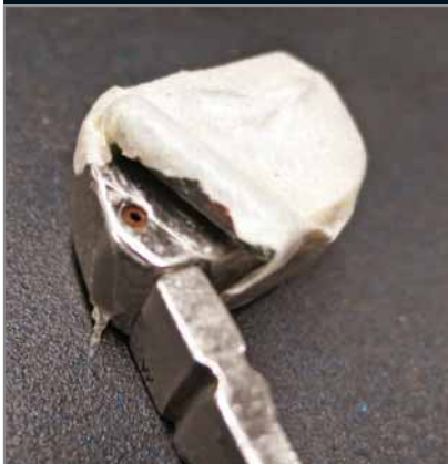
Then we taped it to the salvage yard key. It programmed perfectly with the PIN and the Ross-Tech software.
