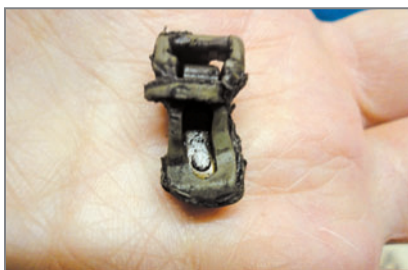
This piece of zip tie wedged itself into the intake valve, holding it open.
