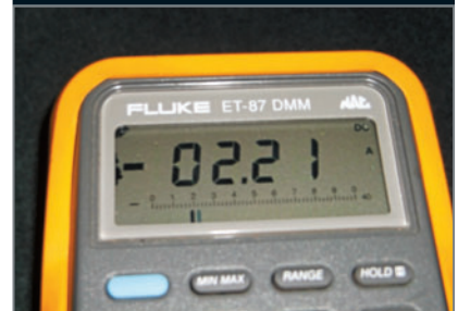
We originally tested the total amperage draw for both heater circuits on the 350Z at the fuse panel behind the left kick panel. Our total amp draw for both AF's heaters read only about 1.4 amps. With the new sensor in place our meter is showing 2.2 amps a few minutes after the engine was started.
