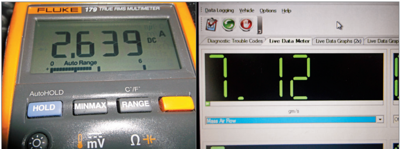
(Left) At a 70°F engine start up, both AF sensors on the 350Z pulled almost 3 amps, but by the time I took this picture the amperage flow had dropped down to 2.64. (Right) Would this reading have caught your eye? The Maxima's MAF varied from 4 to 7.1 g/s. The engine was idling as low as 500 rpms while reading 4 g/s. But the MAF reading went to 7.1 g/s at only 750 rpms. With the car in park we noticed the MAF reading increased faster than the RPMs increased as we revved the engine.
