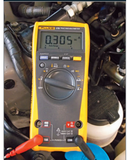
This amp meter reading shows the bad AF sensor heater's reading. Notice the .3 amp as compared to a normal of a little over an amp after the engine had been running for a while.
