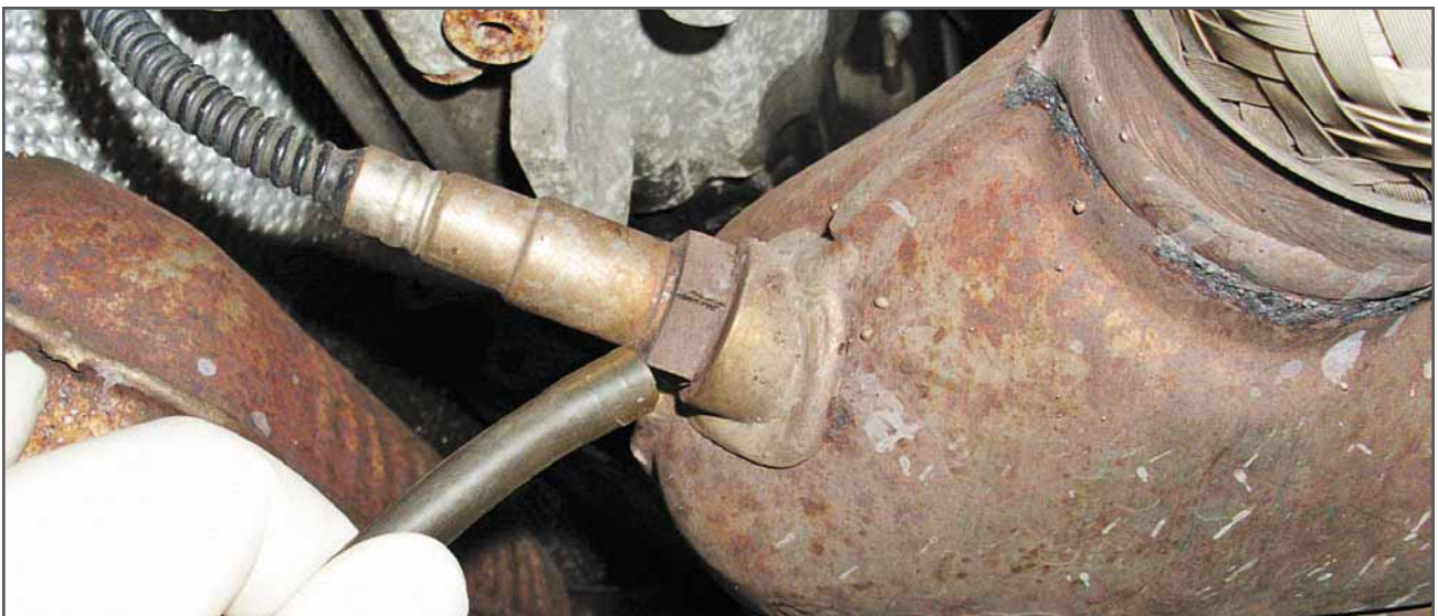
Air leaking upstream of or at the upstream sensor can cause the sensor to read a false lean condition.
