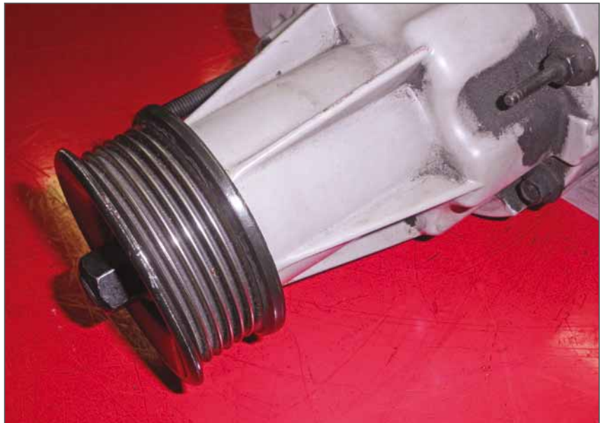
On this Eaton supercharger (GM), if the pulley can be moved up and down or side to side, there is a bearing problem. If the pulley can be rotated several degrees before meeting the resistance of the Roots blower rotors, there are worn out couplers.
