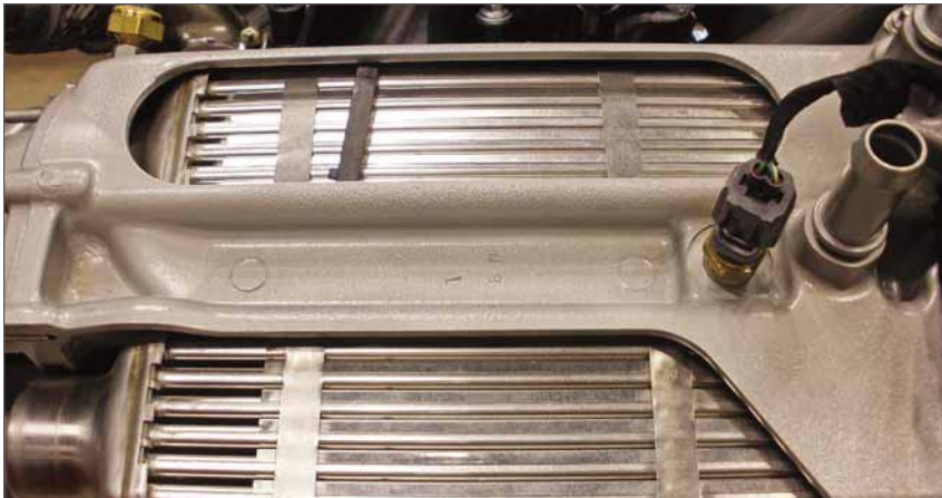
The intercooler is built into top of Ford Powerstroke diesel engine.
