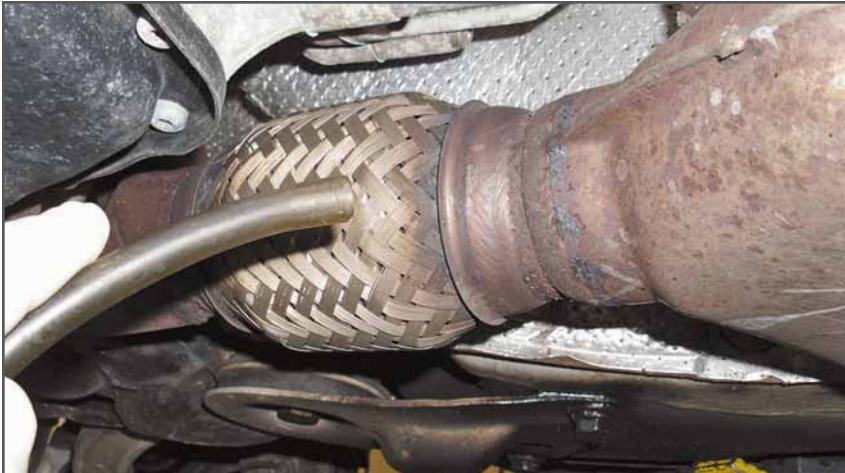
A hose held to the ear is one way to seek exhaust leaks that can cause sensor readings to be off.
