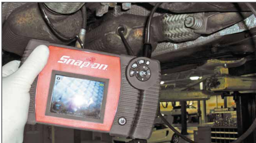
A borescope can be used to inspect the condition of the substrate. Damaged substrate (broken, clogged, melted) means something killed the cat before its time.
