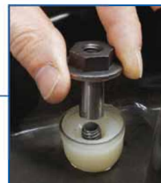
MOOG PROBLEM SOLVER BARREL NUT WITH WASHER MAKES INSTALLATION EASY.
