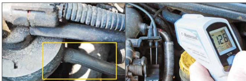
(Left) This third line is also attached to the EGR valve, and feeds exhaust backpressure to the transducer. (Right) One way to tell if an EGR valve is open when it shouldn't be on some applications is to monitor the temperature of the feed tube during a cold engine start. If it heats quickly, odds are good that hot exhaust gasses are passing through it.
