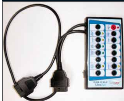
A DLC breakout box is a must have tool for bus troubleshooting.
