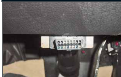
Individual networks may or may not be wired to the DLC.
