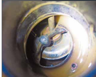
Sometimes the thermostat comes apart like this one did, but usually the spring loses some of its tension and starts opening at a lower temperature.
