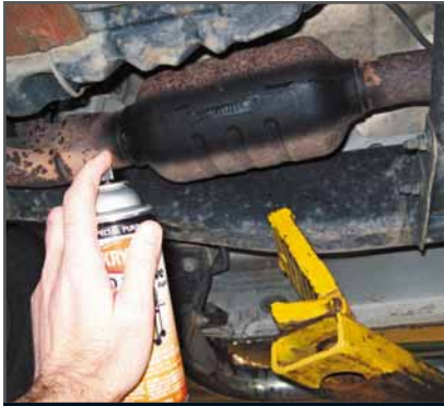
Flat black high-temperature paint can be applied to components to improve temperature accuracy of a thermal imaging camera.
