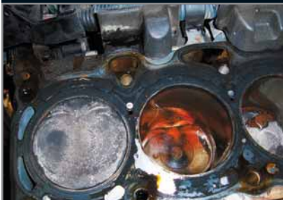
Head gasket leaks can be slow, or occur only after the engine has reached operating temperature. Don't rely on visual signs alone.
