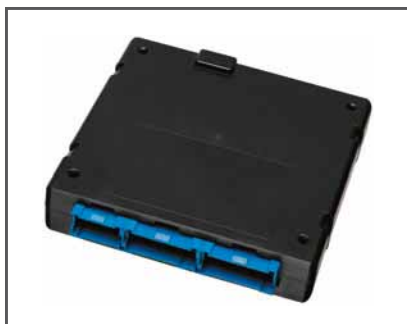
No communications? Multiple networks? Check the gateway module, the network translator.
