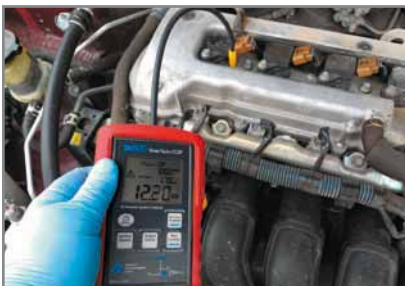
Measuring firing demand and burn time can tell you about more than just the health of the ignition system.
