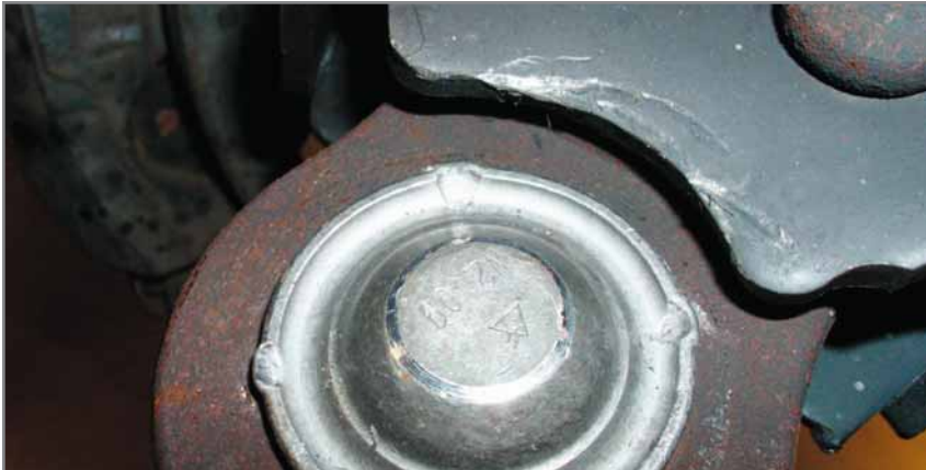
Peened edges or retaining clips aren't designed to make up for sloppy fits.
