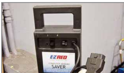
This box has a DLC connector that will keep all the modules going. The old days of a 9-volt battery plugged into the cigarette lighter are long gone.
