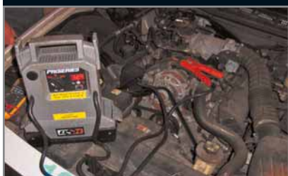
To keep KAM alive, you can connect a jump box or free-standing battery to the alternator B+ post and a good engine ground.
