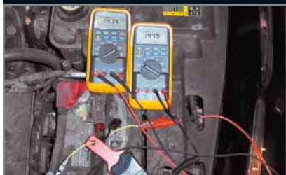
These are identical meters, one using an amp clamp on the millivolt scale and one reading directly using the DC amps scale. Both reading nearly identical.
