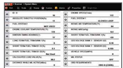
Because this data is from a 2002 model year vehicle, the data is quite limited. In later years, the data stream has increased to a very large PID list.
