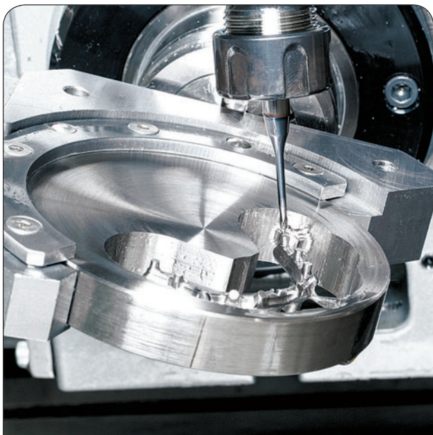
▶ Glidewell utilizes the latest CAD/CAM technology to create passive-fitting milled implant bars consistently.
