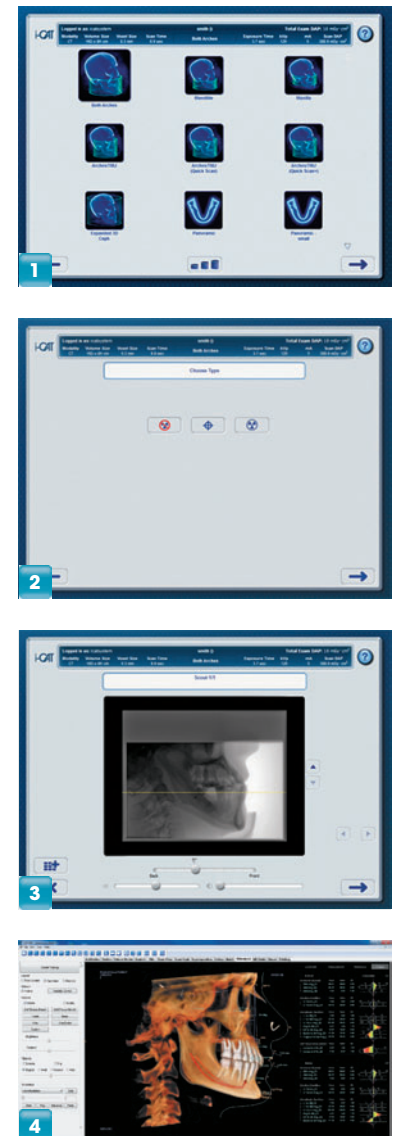
FIGS. 1-4 Select the appropriate scan—traditional 2D i-Pan in large or small or 3D scan in various diameters, heights and resolutions—by touching the proper image on the screen (Fig. 1). Once the patient is in position, the next screen allows for a Scout, Dry Run, or the actual Scan capture (Fig. 2). With the “Scout” image, we are able to reposition the patient and to decrease or increase the height and position of the scan, as needed, then take the actual scan (Fig. 3). Within Tx STUDIO, I have access to a collection of diagnostic and treatment tools specific to orthodontics. There are also tools specific to other procedures such as airway and implants (Fig. 4).
