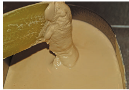
Figs. 7a and 7b Measurements for an average model are 150gr of stone to 50 mL of Wonderadmix. Consistency of stone when mixed for models or capping is smooth, creamy and easy flowing. Slight vibration immediately causes it to flow.
