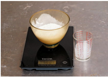
Figs. 7a and 7b Measurements for an average model are 150gr of stone to 50 mL of Wonderadmix. Consistency of stone when mixed for models or capping is smooth, creamy and easy flowing. Slight vibration immediately causes it to flow.
