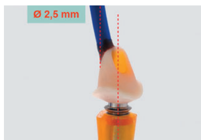
Fig. 6 A 2.5 mm sprue was attached to a circular area of the wax-up, being certain to keep the sprue parallel with the screw access channel.
