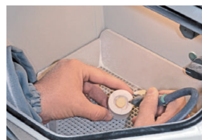
Fig. 8 The restorations were removed from rings, divested and immersed in Invex Liquid to remove the reaction layer.
