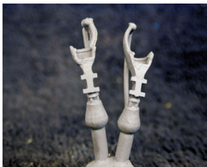
Fig. 4 Sprue, invest and cast the housing patterns with the lingual arms.
