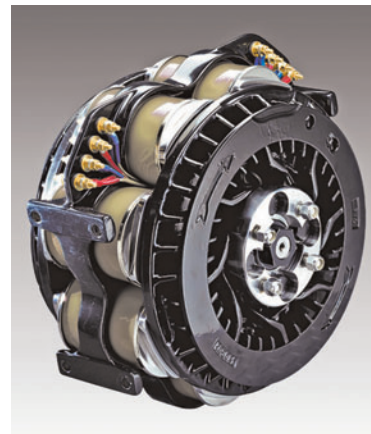
This Dynojet eddy current load absorption unit is ideal for testing motorcycle engines because of its quick response and loading capabilities. The electromagnetic coils can be seen next to the heat absorption rotor. The rotor looks like a disc brake for a car and has large cooling fins and passages to dissipate heat created by a loaded engine.
