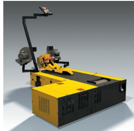
This Dynojet 250i load control (eddy current) dynamometer can hold engine speed steady at any throttle opening. The dyno can measure up to 750 horsepower at speeds of 200 mph. It can also be configured to run sweep tests like an inertia dynamometer. This type of dynamometer is available in a portable design (pictured) or for in-ground installations.
