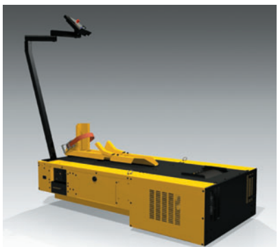
The Dynojet 200i from Dynojet Performance is an inertia type chassis dynamometer that provides a quick way for motorcycle dealers and independent repair shops to verify repairs and diagnose a variety of performance problems. It comes with an atmospheric module that provides a correction factor to ensure consistency between dyno runs made under varying conditions.
