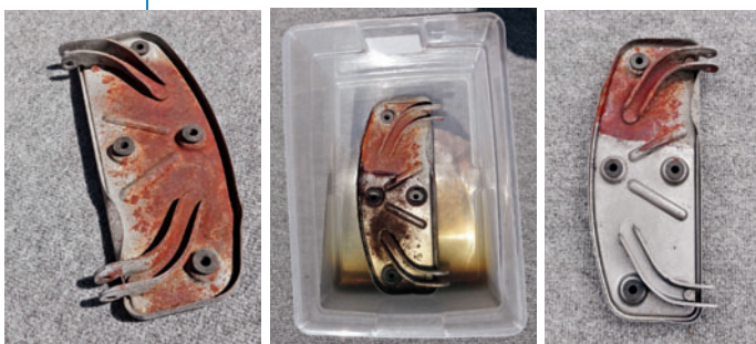
From left to right: A Harley-Davidson floorboard with 40 years' worth of rust; after a two-hour soak in Metal Rescue; after four hours of soaking in Metal Rescue.
