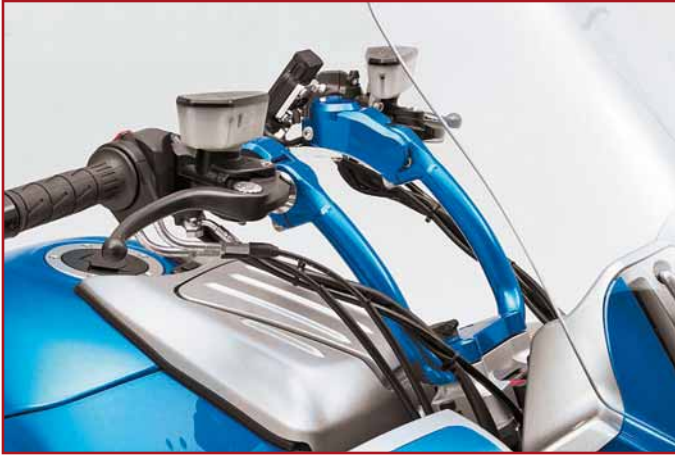
HeliBars Horizon ST Multi-Adjustable Handlebar Replacement System, this one on a 2012 Kawasaki C14
