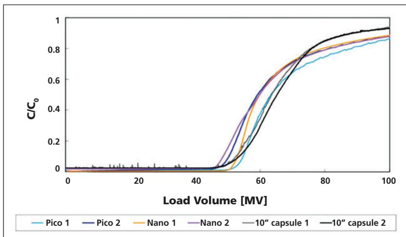
up to 1000 MV was monitored at a constant pressure of 3 bar using a balance.
