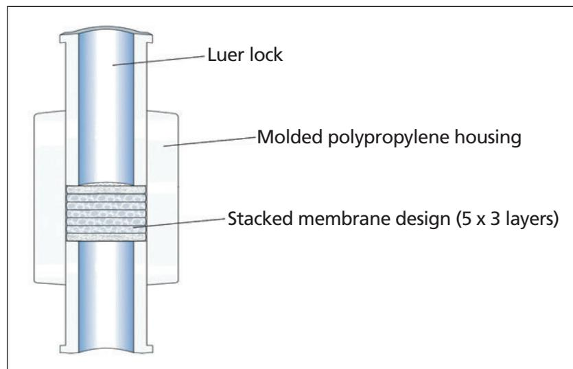
(Sartorius Stedim Biotech GmbH, Göttingen, Germany) with 15 layers, 36.4 cm<sup>2</sup> total surface area, and 1 mL membrane volume was used as a reference device (see **Figure 1**). The Sartobind nano has a radial flow and is constructed in the same way as process scale
