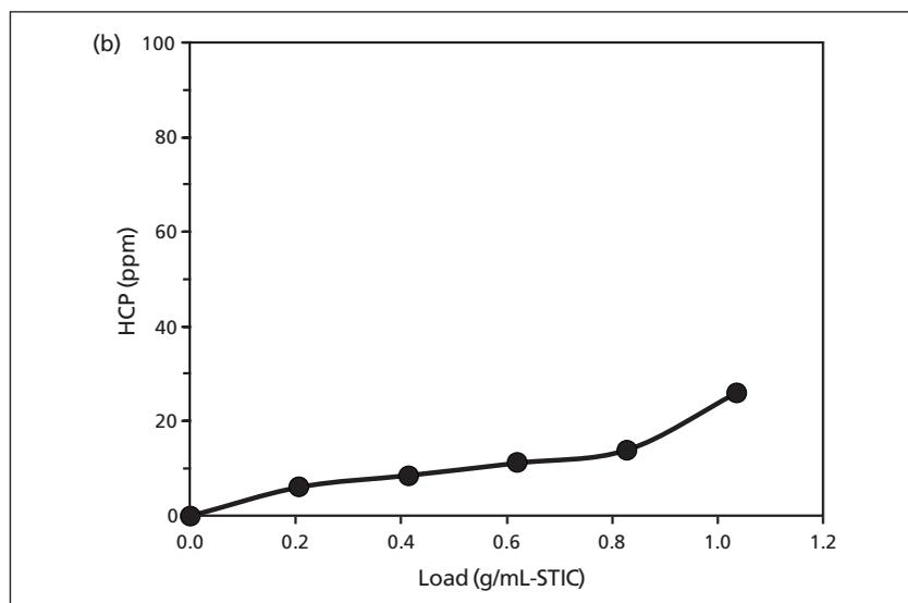
**Figure 4:** Determination of dynamic loading capacity of Mab-S monoclonal antibody on Sartobind salt tolerant interaction chromatography (STIC) in terms of residual host cell protein (HCP) level. Buffer condition: pH 7.0, 9.53 mS/cm; Mab-S mAb concentration: 12.6 mg/mL; Impurities in the starting materials: high molecular weight (HMW) species: 0.9%, HCP: 212 ppm; flow rate: 10 mL/min.
