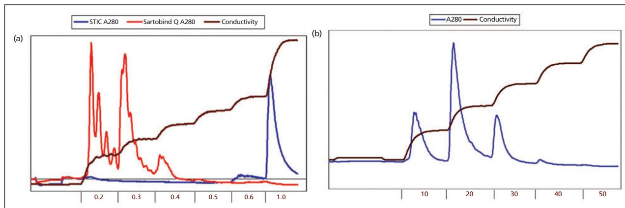
**Figure 3:** Dynamic binding capacity of host cell impurities by Sartobind STIC. a) Host cell proteins breakthrough curve with host cell protein (HCP) spike-in. b) DNA breakthrough curve with representative immunoaffinity eluate.
