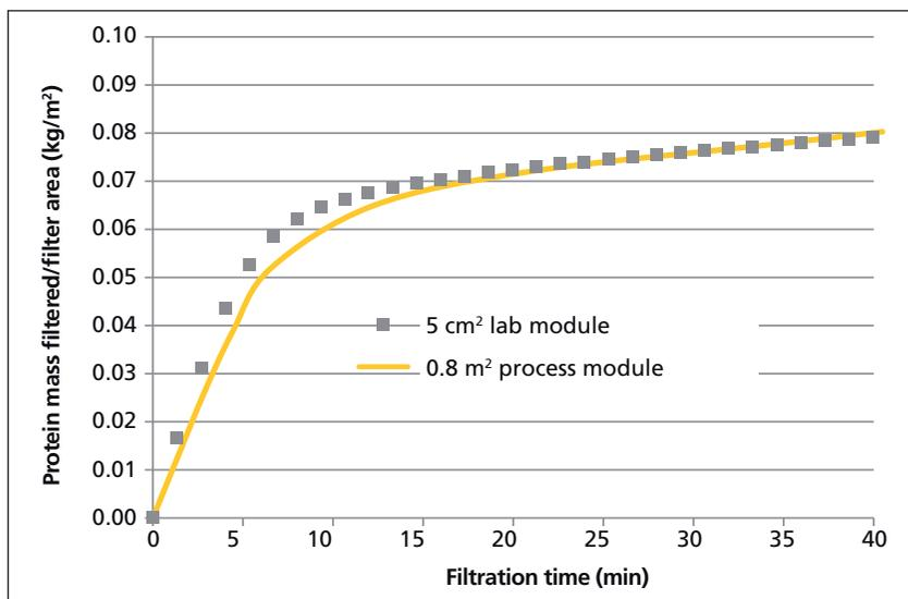
**Figure 4:** Virosart HF laboratory modules were challenged with a 10-20-g/L monoclonal antibody solution (pH 6-7, conductivity 4-8 mS/cm) spiked with 0.5% MMV. Experiments were carried out at constant flux at 120 L/m<sup>2</sup>h. The membrane was challenged with up to 7.4-kg antibody/m<sup>2</sup> resulting in a permeability decay of more than 70%. A log reduction value of greater than 5 was achieved in both spike trials (Run B and Run C).
