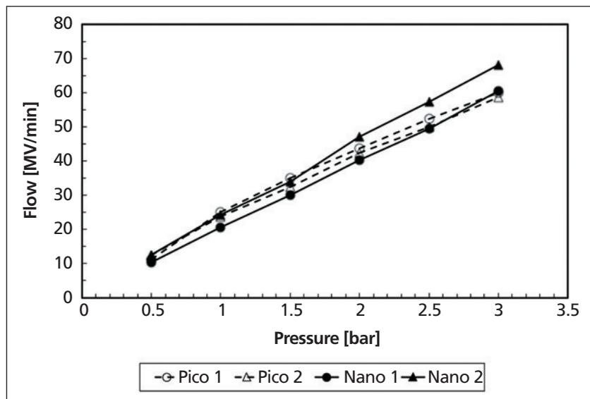
**Figure 4:** Filtrate flow rate at 3 bar constant initial pressure during loading of 20 g/L  $\gamma$ -globulin protein solution. MV is membrane volume.
