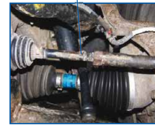
NOTE BROKEN SWAY BAR LINK
