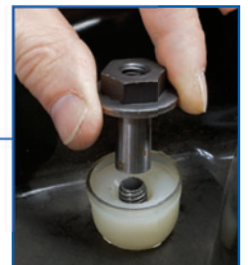
MOOG PROBLEM SOLVER BARREL NUT WITH WASHER MAKES INSTALLATION EASY.
