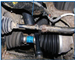
NOTE BROKEN SWAY BAR LINK
