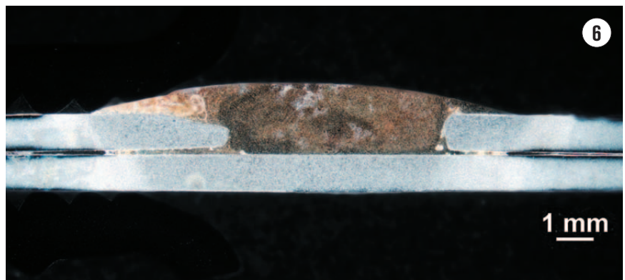
GAS METAL ARC BRAZED JOINTS
