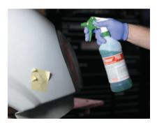
CLEAN AND PROTECT DAMAGED COMPOSITE
