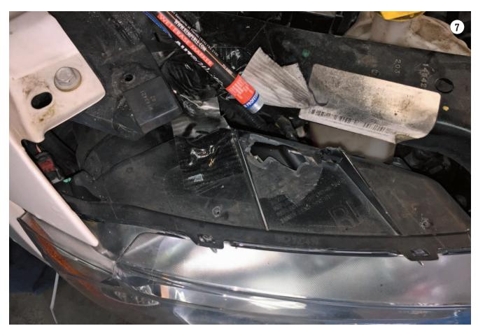
stripped in the holes and did not bite the metal properly. The radar assembly was compromised because it would never be able to sit in the proper position as designed. The bumper supports looked similar (Figure 5) and mounted correctly, but the one for the radar unit was much more money and had nuts welded on the inside to accommodate the radar assembly.
