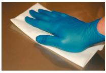
NORMAL PREP WORK PRODUCES STATIC ELECTRICITY on parts that can attract particles, which in turn create imperfections when finishes are applied.
