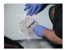
ELIMINATE AIR POCKETS IN REPAIR AREA
