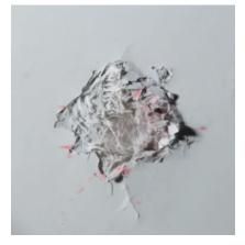
**DAMAGED COMPOSITE TO REPAIR**
