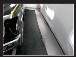
Netting can be used on the booth floor by securing with duct tape. Will trap overspray and dirt from getting in wet paint.
