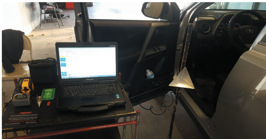
HERE IS A TOYOTA TECHSTREAM SCAN TOOL and the target for an Adaptive Cruise Control aiming procedure. ACC and BSM tool are the same for some Toyotas.
