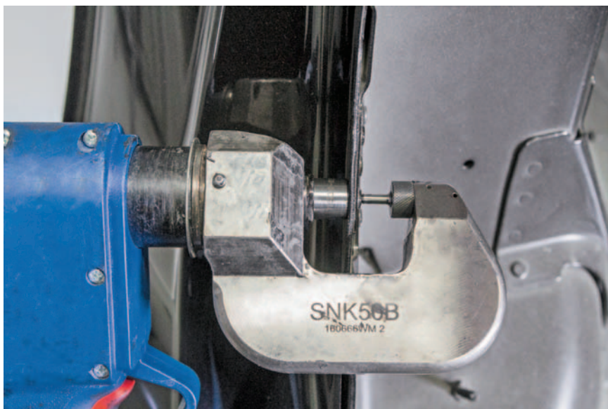
FACTORY-INSTALLED SPRs will often be replaced with blind rivets during repair.
