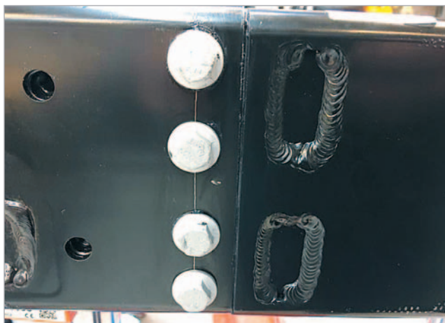
AUDI Q7 lower front aluminum rail sectioning bolt bonding
