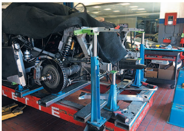
PORSCHE 911 (996) rear structure repair on a Celette.
