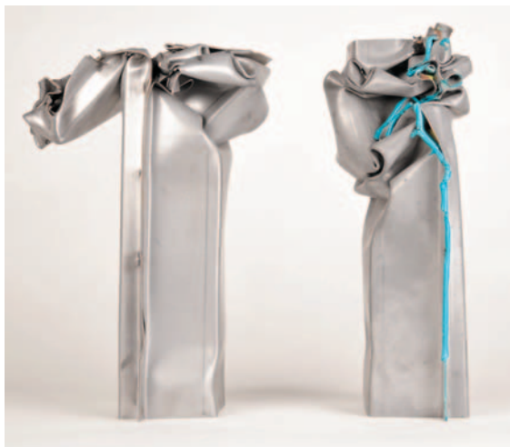
CRASH-DURABLE ADHESIVES ensure that structural parts such as these frame rails properly absorb energy.
