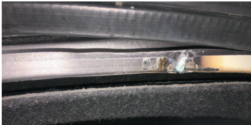
AN EXPOSED WELD with no corrosion protection was hidden by the weather strip.
