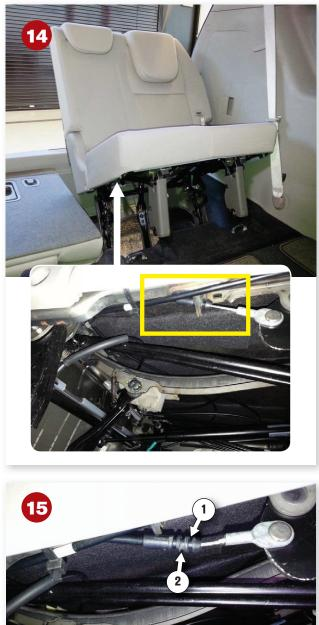
**15.** Use a long needle nose plier to remove the cable adjuster from the holder. Note: The default setting for the cable adjuster is slot two 2. If there is excess tension in the seat release mechanism, reinstall the cable adjuster using slot one 1.
