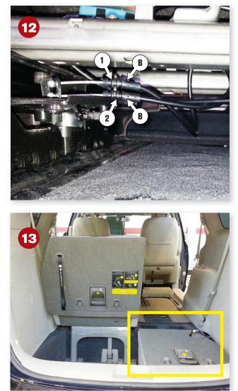
**12.** Use a long needle nose plier to remove the cable adjuster from the holder. Note: The default setting for the cable adjuster is slot 2. If there is excess tension in the seat release mechanism, reinstall the cable adjuster using slot 1.
