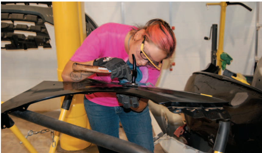
APPRENTICE CHRISTINE NEWMAN uses a hammer and dolly on fender damage.
