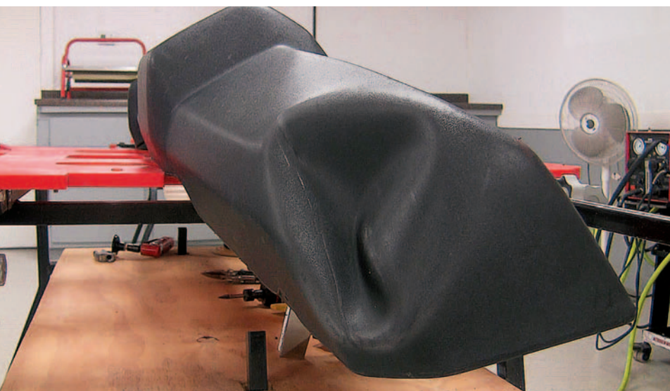
THIS JEEP WRANGLER blow-molded bumper has suffered a deep dent in the corner. To push the dent out, an access hole will have to be cut on the backside.
