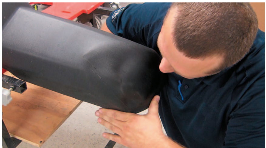
PUSH THE DENT out with a blunt tool. Push up on the low spots and shrink the high spots while the plastic is hot.
