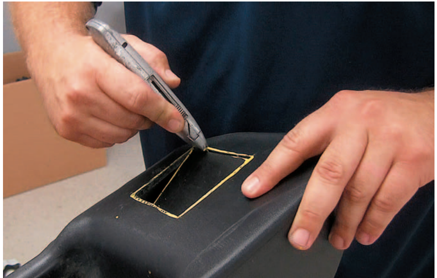
CUT A HOLE on the backside to allow access to push the dent out from the back.
