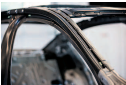
2016 BMW 7 SERIES (G12) upper roof rail, front header and inner B-pillar reinforcements CFRP
