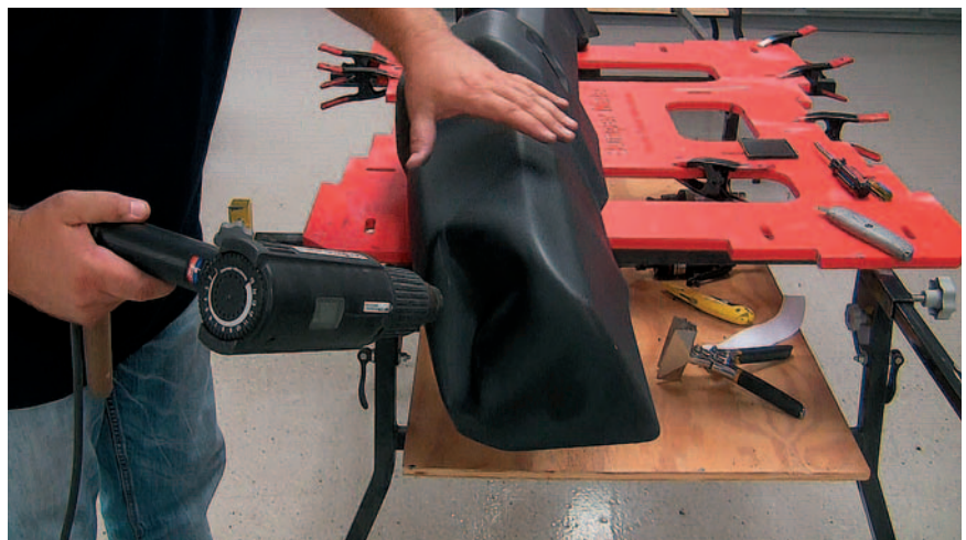
HEAT THE BUMPER carefully with a heat gun to soften the plastic.
