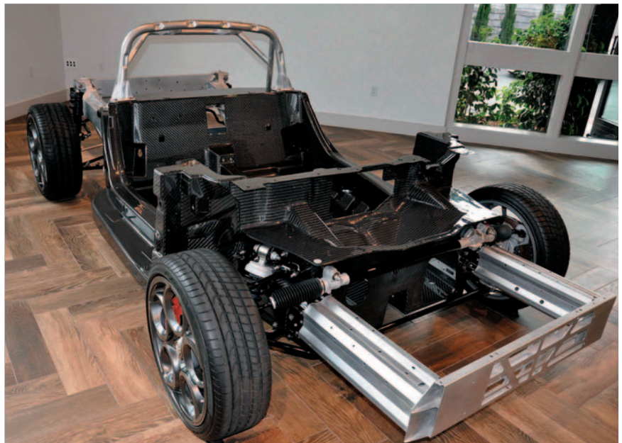
ALFA Romeo Spider 4C body-in-white
