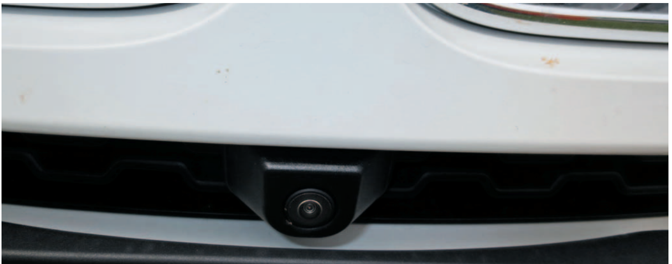
AFFORDABLE VEHICLE AND LUXURY VEHICLE – both vehicles have advanced safety systems and use cameras located in the front grill.
