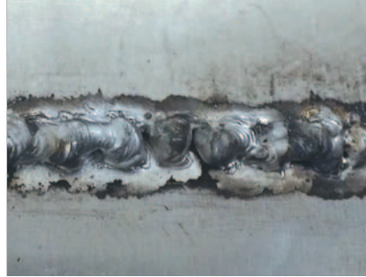
EXAMPLE WELDING CURRENT SYMPTOMS: Amperage Too Low (left), Amperage Too High (right).
