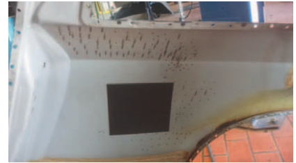
QUARTER PANEL, WAVY PANEL back-side with excessive burns and no corrosion protection applied
