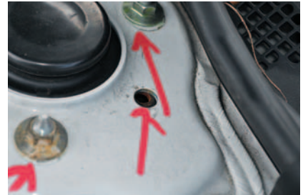
MISALIGNED strut mounting bolts
