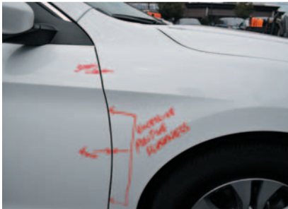
PANEL GAP ISSUES on vehicle with misaligned strut tower
