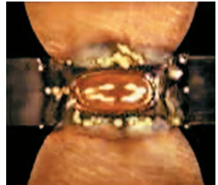
A SPOT-WELD cross section
