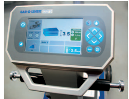
CTR7 MMI showing weld results
