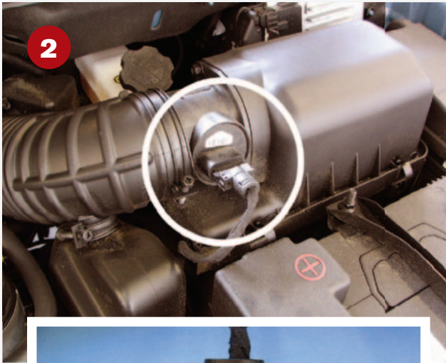
Gray lock tab shown here in the released (outward) position.
