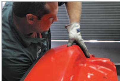
Pushing the dent out
