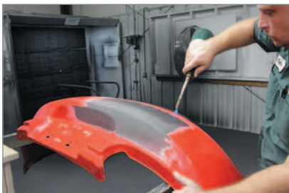
Flame treating to remove fuzz
