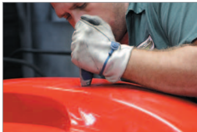
Pushing down the high spots
