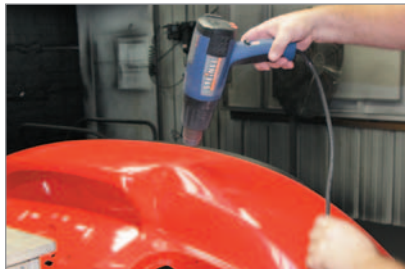
Heating around the dent
