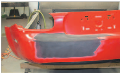
Dent removed, ready for finishing
