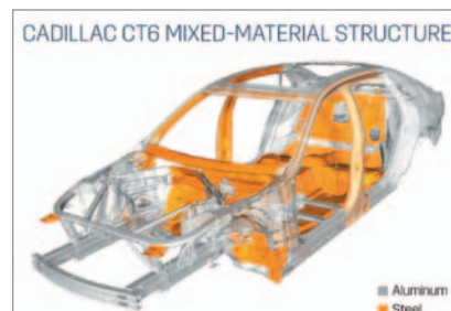
The Cadillac CT6 mixed material structure uses advanced aluminum and steel to save 218 pounds.
