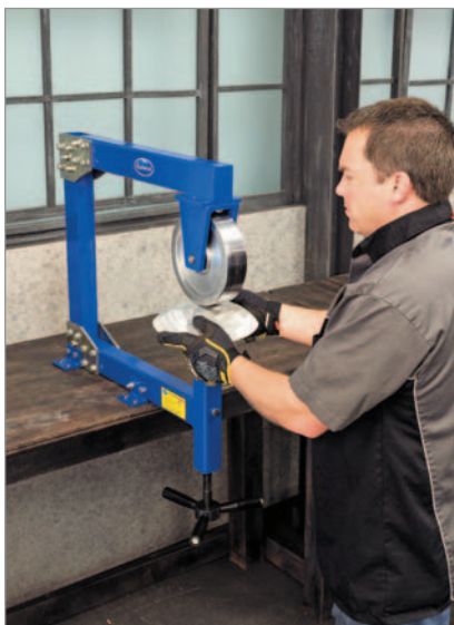
The more difficult aspects of learning fabrication include mastering tools such as this bench-top English wheel.
