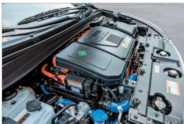
Hyundai Tucson Fuel Cell Engine Compartment
