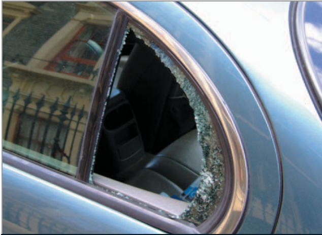
Note the broken glass surrounding the repair area. All of this glass will need to be removed, and the area will require surface protection during the repair.
