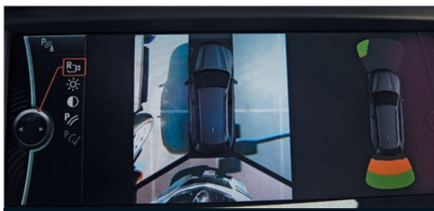
2014 BMW X5 Diesel while parking. Some vehicles offer an overhead view of the vehicle in both an animated picture of the vehicle and its surrounding objects and an actual camera picture as well.
