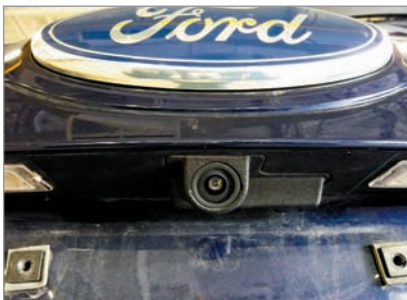
Rearview camera of 2012 Ford Edge. Starting May 1, 2018, the NHTSA has ruled that all vehicles manufactured for use in the United States under 10,000 lbs must come equipped with back-up cameras installed. These will likely be the most common collision avoidance system you will encounter in the shop.
