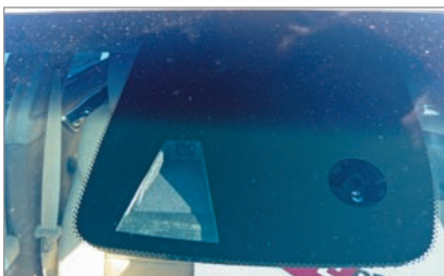
Image of 2013 Cadillac Front Camera Module. No recalibration of the Cadillac Front Camera Module was required when replacing the windshield as long as it was remounted correctly. In fact, it doesn't require recalibration even when reprogramming the original module, only when replacing.
