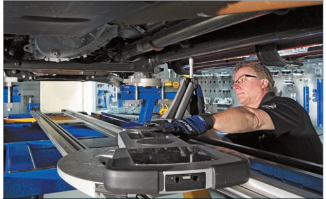
On today's collision restoration, millimeters now make a huge difference in lower body and suspension points. The vehicle must perform and maintain the same level of safety to the occupants as before the repair.
