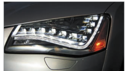
Most AFL systems will require some type of calibration with a capable scan tool when replaced and since LEDs are not available separately, the entire assembly must be replaced as a unit.
