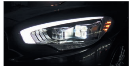
Most newer vehicles are equipped with Adaptive Front Lighting Systems that utilize LEDs to manipulate the direction and area illuminated. This is a 2015 Kia K900.
