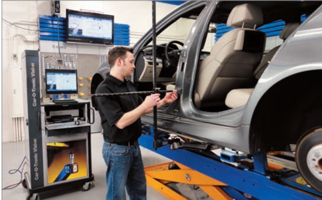
Upper body digital measurement assures the job is done right the first time. Time can be saved by assuring perfectly located door hinge mounting points and panel gap alignment.
