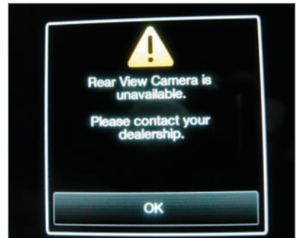
Ford Edge with defective rearview camera. This is what the customer will usually see on the display screen when the vehicle is put into reverse and there is a fault in the rearview camera system.
