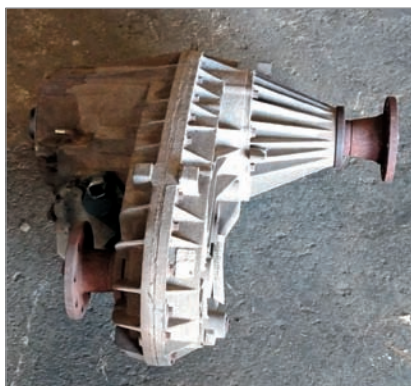
A typical 4WD transfer case bolts to the back of a transmission and splits power to the front and rear axles as commanded.
