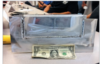
4mm cast to 2mm plate.
