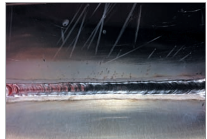
2mm to 2mm plate 300mm long open butt weld.
