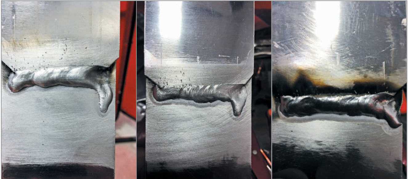
Fillet 3mm chilled cast to 3mm chilled cast.
