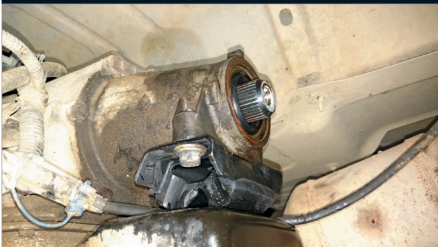
The more common type of output is a slip yoke. This one is on a 2002 Chevrolet 2500 Silverado. The slip portion in the tail housing serves the same purpose as the slip section on a fixed yoke driveshaft.
