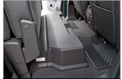
Examine carpeting and areas under the seats for water stains, dampness and rust.
