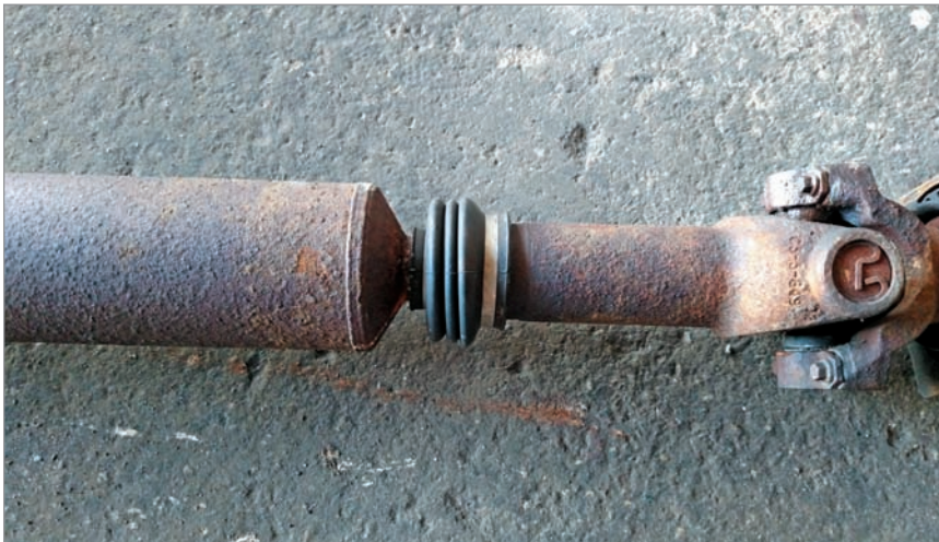
Typical fixed yoke transmissions will incorporate a slip section on the driveshaft to account for suspension travel and drive train movement.
