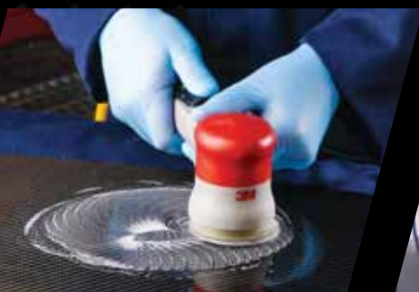
STEP 2: Sand down the nick and surrounding area.
