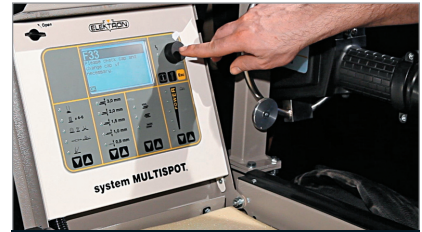
Automatic spot welders are becoming more common in collision repair shops. These welders continually detect metal composition and material thickness through electrical impedance and automatically adjust current levels, clamp pressure and weld time on the fly.
