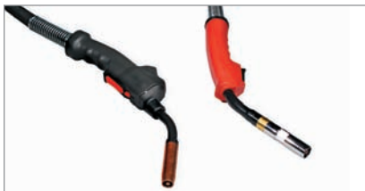
Advanced MIG/MAG welders are available with a push-pull torch (left) that maintains constant, uniform tension on soft aluminum wire. Traditional MIG/MAG torches are fed solely by a feeder in the base unit, which can lead to wire tangles.
