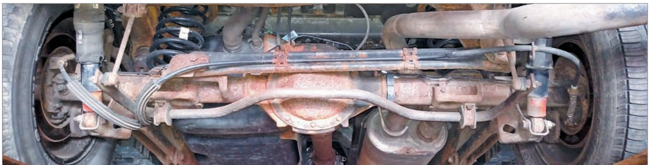
Typical solid axle configuration from a 2004 Cadillac Escalade at Pete's Garage Inc.
