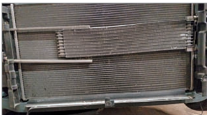
This cooler from a 2004 Chrysler minivan has separated from its mount during a collision. It's tricky to spot but if let go, the long term vibrations will cause cooler or related component failures.
