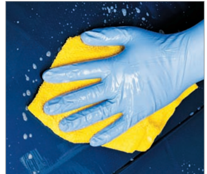
Begin any filler repair by using hot water and soap to clean the area then follow with a residue remover to eliminate any remaining contaminants.
