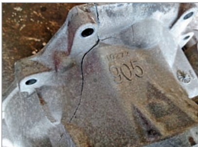
Broken Bell housing/case in a 2004 Chevrolet Monte Carlo
