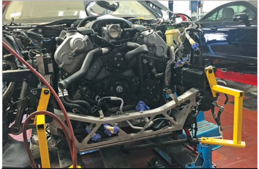
Porsche 970 front lower uni-rail sectioning
