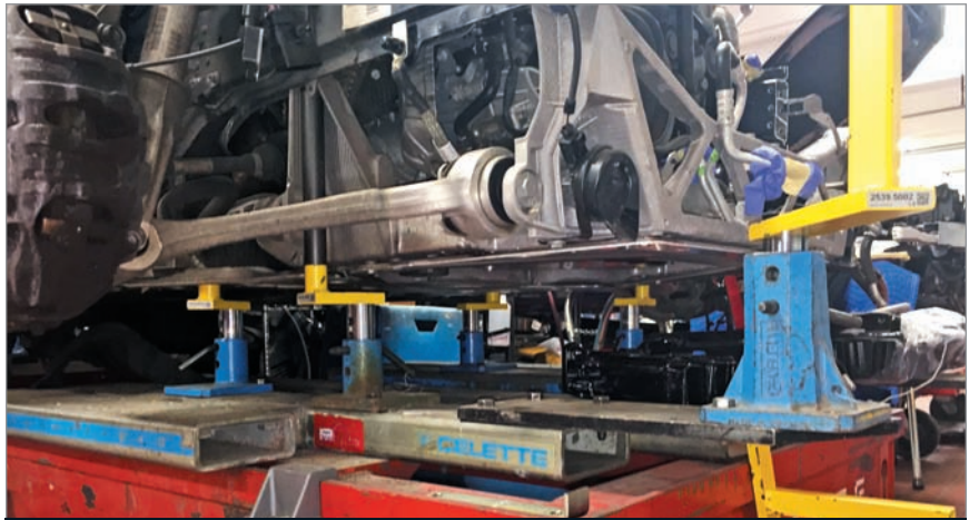
Porsche 970 front lower uni-rail sectioning
