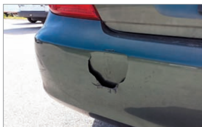
Adhesives have improved to the point where they can handle a range of plastic and metal repairs that once would have called for a replacement part.
