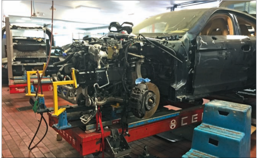
Porsche 970 front lower uni-rail sectioning
