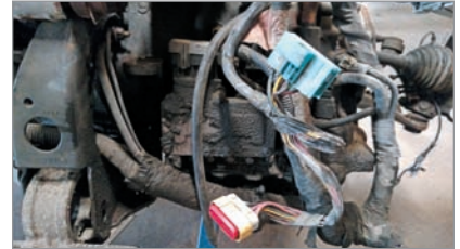
Wire harness, solenoid packs and ECM are often exposed and easy to damage in a collision, visual inspection can often identify damaged components.
