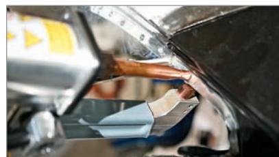
In the weld bonding process, squeeze-type resistance spot welding (STRSW) forms a welded attachment that replicates the original assembly.
