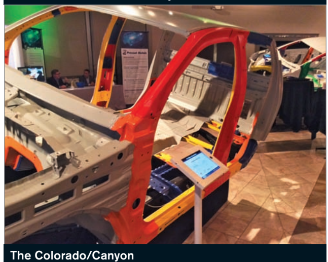
The 2015 GM Colorado/Canyon cab structure
