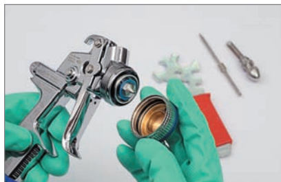
During a thorough cleaning, the gun needs completely disassembled, with the cap pulled.
