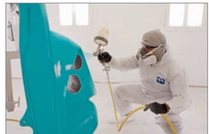
Correct spraying distance is 4-6 inches from the vehicle.
