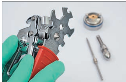
Repairers need to make sure a spray gun is fitted with the correct tip for the product being applied.
