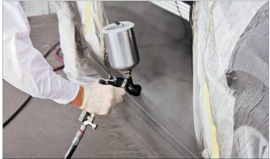
A poorly maintained spray gun costs a shop twice — in poor finishes that must be redone and in reduced service life.
