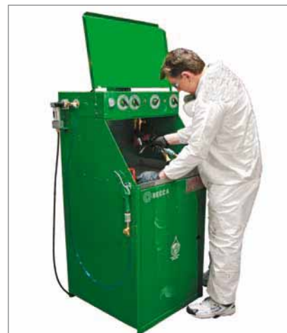
Gun cleaning machines provide quicker and more thorough cleaning of spray guns than manual cleaning, along with reducing the release of VOCs.
