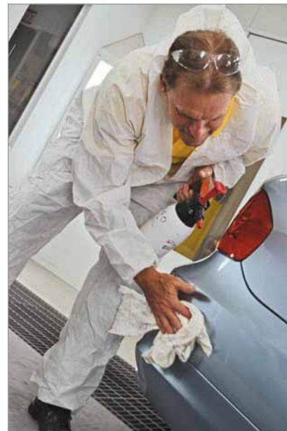
Clean vehicles twice before they are painted — first when they enter the shop and again at the beginning of the prep work.
