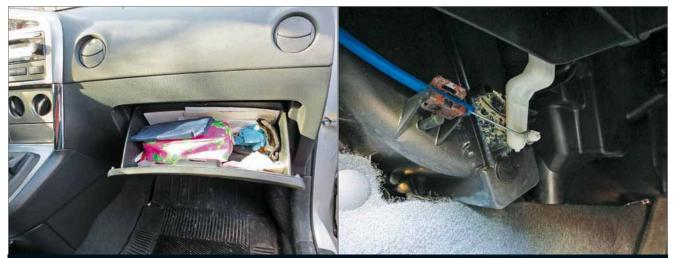
(Left) Glove boxes are often full of things that could potentially escape out over the top and end up interfering with the doors and linkages that control the cabin temperature. (Right) HVAC control cables tend to get knocked off or moved out of adjustment by the vehicle's floor mats — especially winter ones that aren't shaped to the floor.
