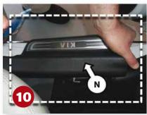
Move the front seat as far forward as possible and use a plastic prying tool to remove the front door threshold panel (M).
