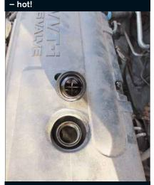
If you suspect an internal coolant leak is causing a noheat situation, take a look at the engine oil filler cap. If it's covered in foamy white goo you may be correct (this one pictured is fine).
