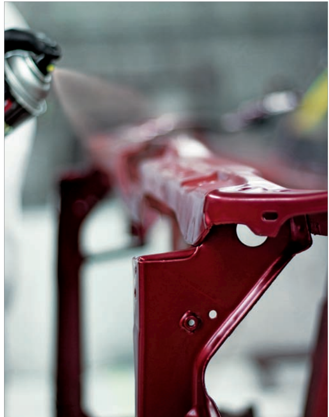
1K HS Clear being applied on a radiator support during the final step of SEM's labor saving OEM Refinishing System.
