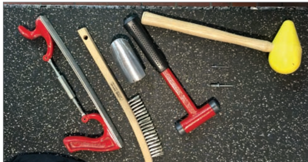
From right: Plastic hammer, rubber hammer, steel dolly, stainless steel wire brush and file
